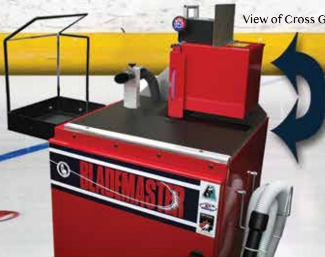
Head pivots between cross-grind & finishing positions
